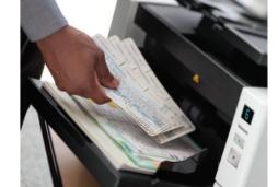
SurePath Paper Handling automatically adjusts for a variety of document sizes and thicknesses.
